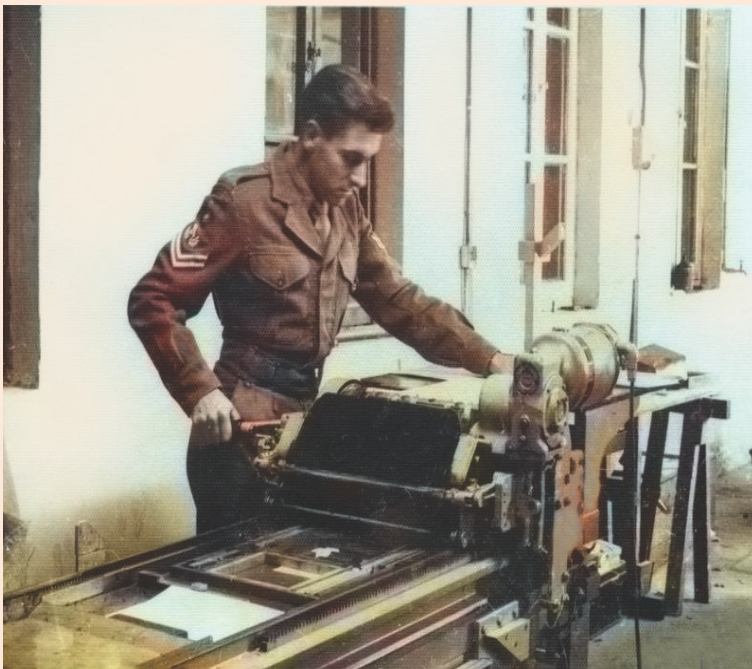
Printing the map place names on a proof press
